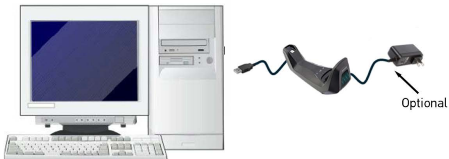
Figure 13 - Connecting to the Host RS-232
