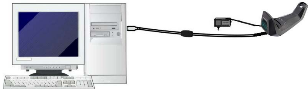
Figure 13 - Connecting to the Host RS-232
